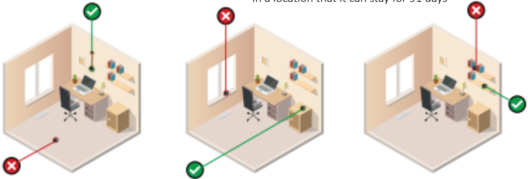
Figure 4. Potential testing locations in an office. Locations that are appropriate (✓) for radon testing and locations that are not appropriate (✗) for radon testing are indicated.
